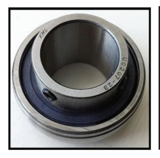
In many **KML** bearing styles the original seals and/or flingers are reinstalled after the solid lube is cured in the ball cavity. This extra sealing protection increases the service life of the bearing. It is not uncommon to double or triple the operating life of the bearing in the original application due to the superior performance of the solid lubricant coupled with labyrinth sealing systems.
